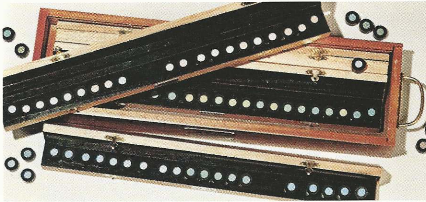
Farnsworth–Munsell 100 hue test. Observers are instructed to order the colored caps in hue. Observers with color-vision deficiencies will make systematic errors, enabling diagnoses.
